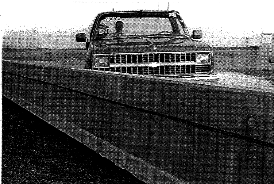
Figure 15. Vehicle/bridge railing geometrics for test 7069-4.
